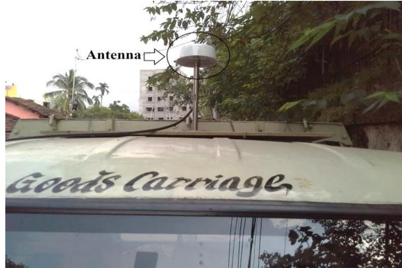
Pick up vehicle with external GNSS antenna
