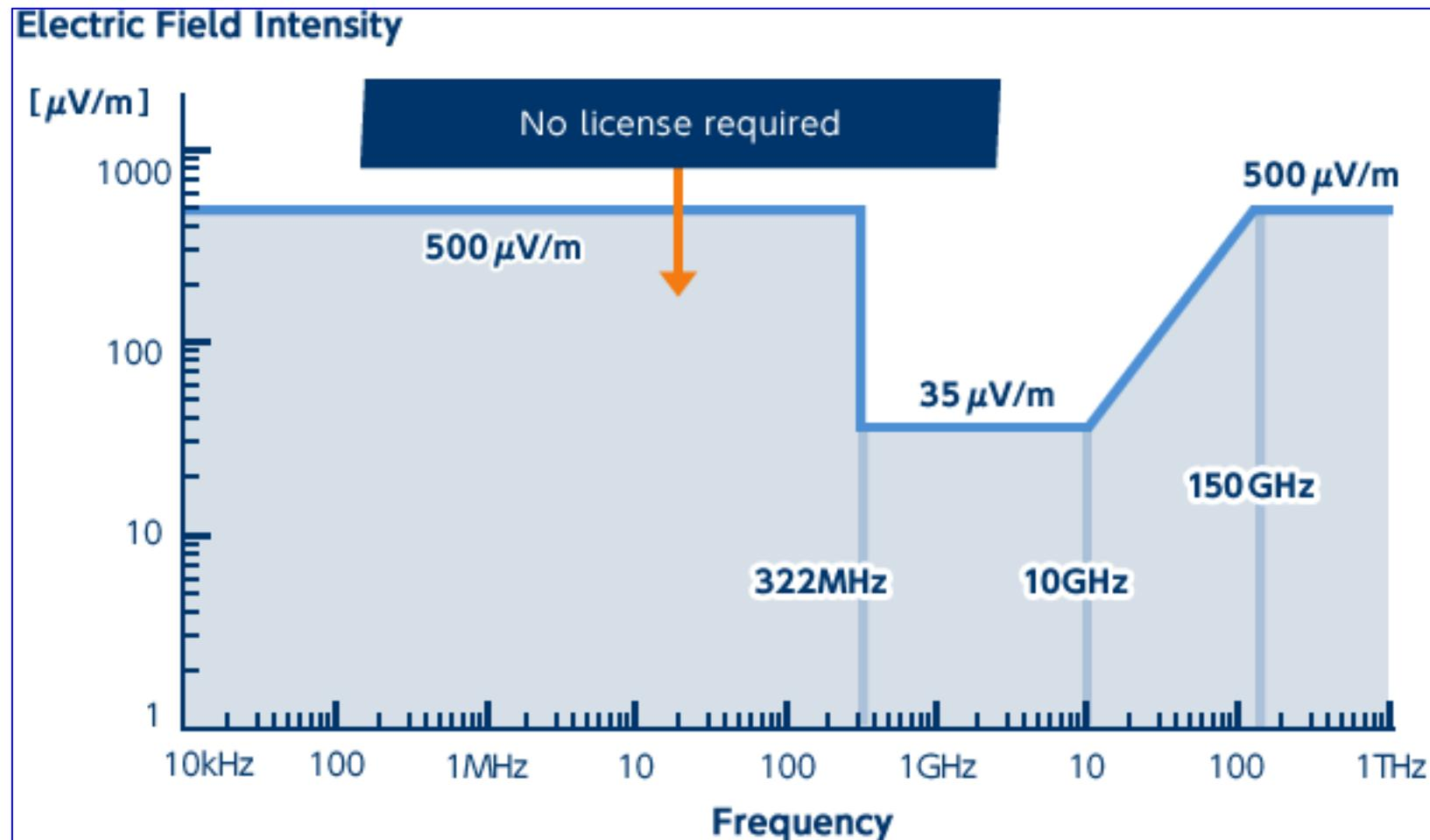
Maximum Field Intensity of RF signal at 3m for License Free operation in Japan
