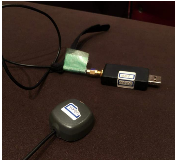
Figure 1: Low Cost M8T u-blox receiver for logging GNSS Data
