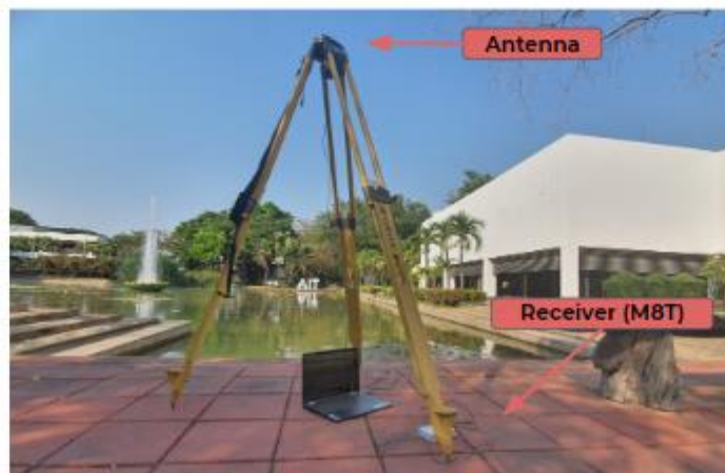
Figure 2. Fieldwork set-up for data collection (Static)
