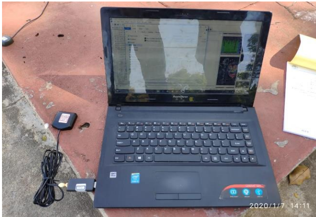
Figure 1.5 Stationary Point Positioning Using single Band Receiver( M8T )
